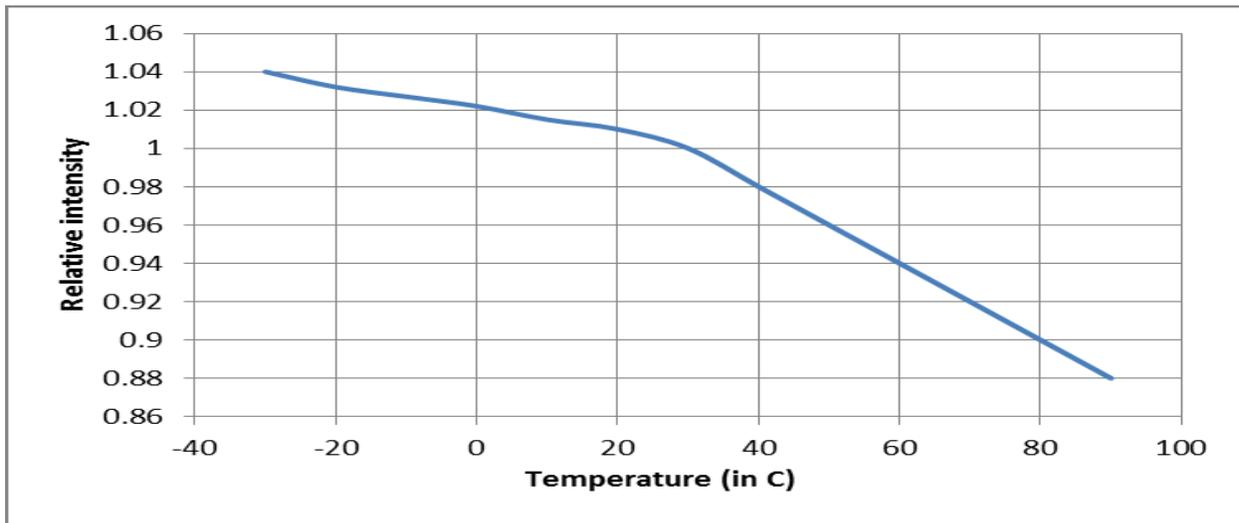
**Figure 4: LED relative intensity vs Temperature**
