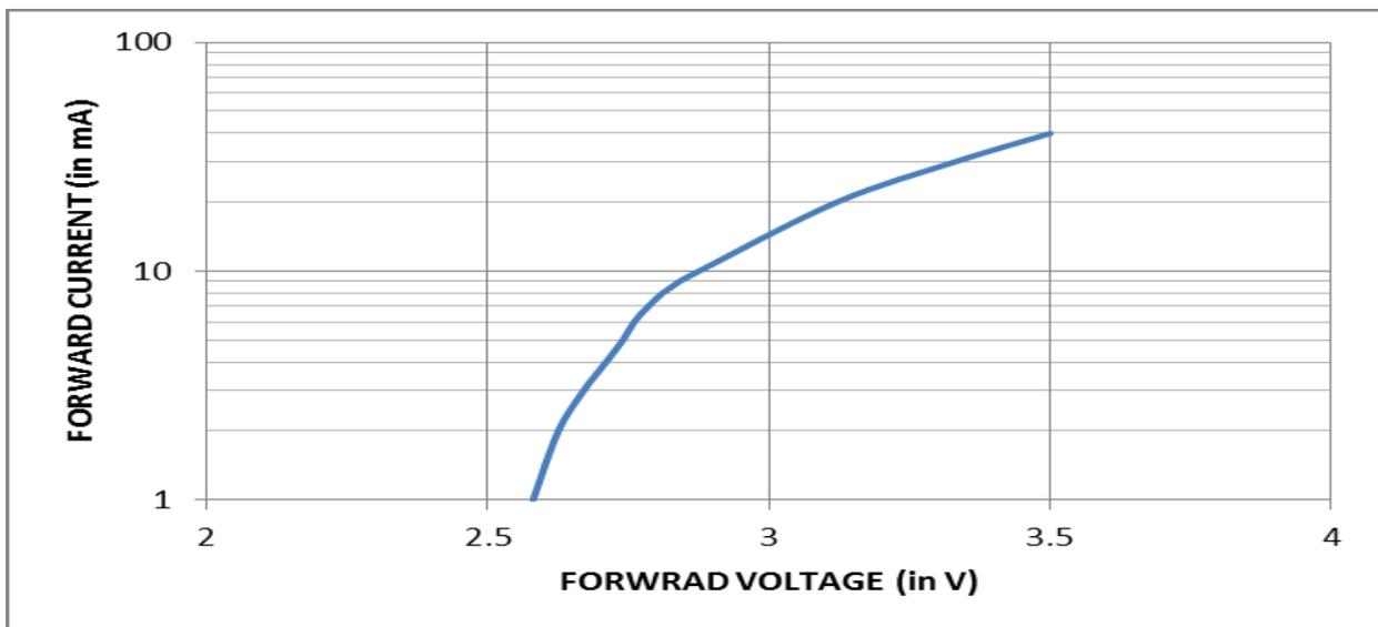
**Figure 2: LED forward voltage vs. LED Forward current**
