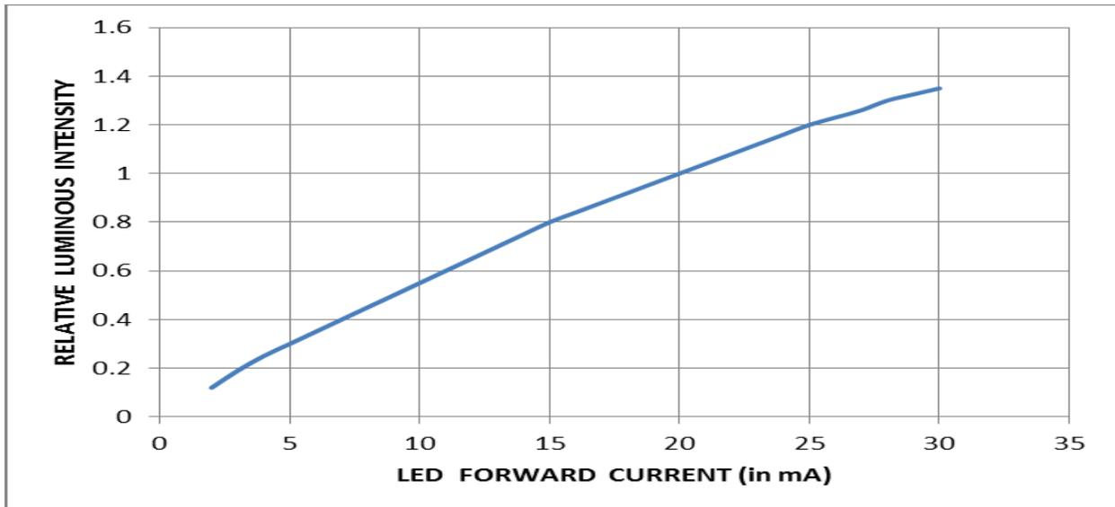
**Figure 1: LED Relative intensity vs. Forward current**
