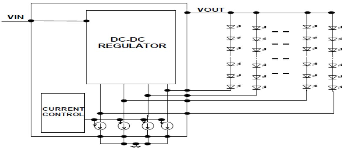
**Figure 3: Typical WLED backlighting system**
