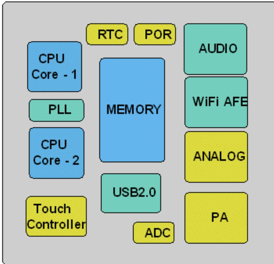
Figure 1: Example of sub systems in a SoC. Power requirements will be different for all these sub systems.
